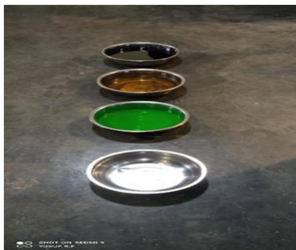
Figure 2. Quenching media used in the hardening process.
